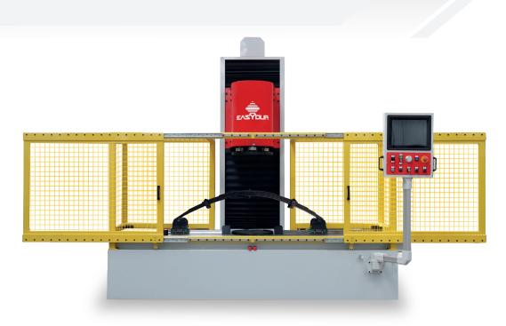
The **Arco model leaf spring testing machine** is the ideal solution for performing **compression** and **bending tests** on leaf springs mainly intended for railway and automotive applications.
